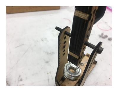
4. Hold the **catapult arm(3)** where you want to put it, then slide the **pivot bolt(7)** through a hole in the upright pieces and the arm. If this is the first time you're using the catapult, try the hole on the uprights and the hole on the arm, shown in the picture above.
