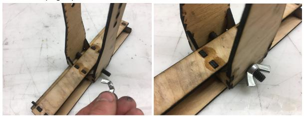
3. Screw **assembly wing nut(5)** onto the end of the bolt to secure the upright pieces to the base.
