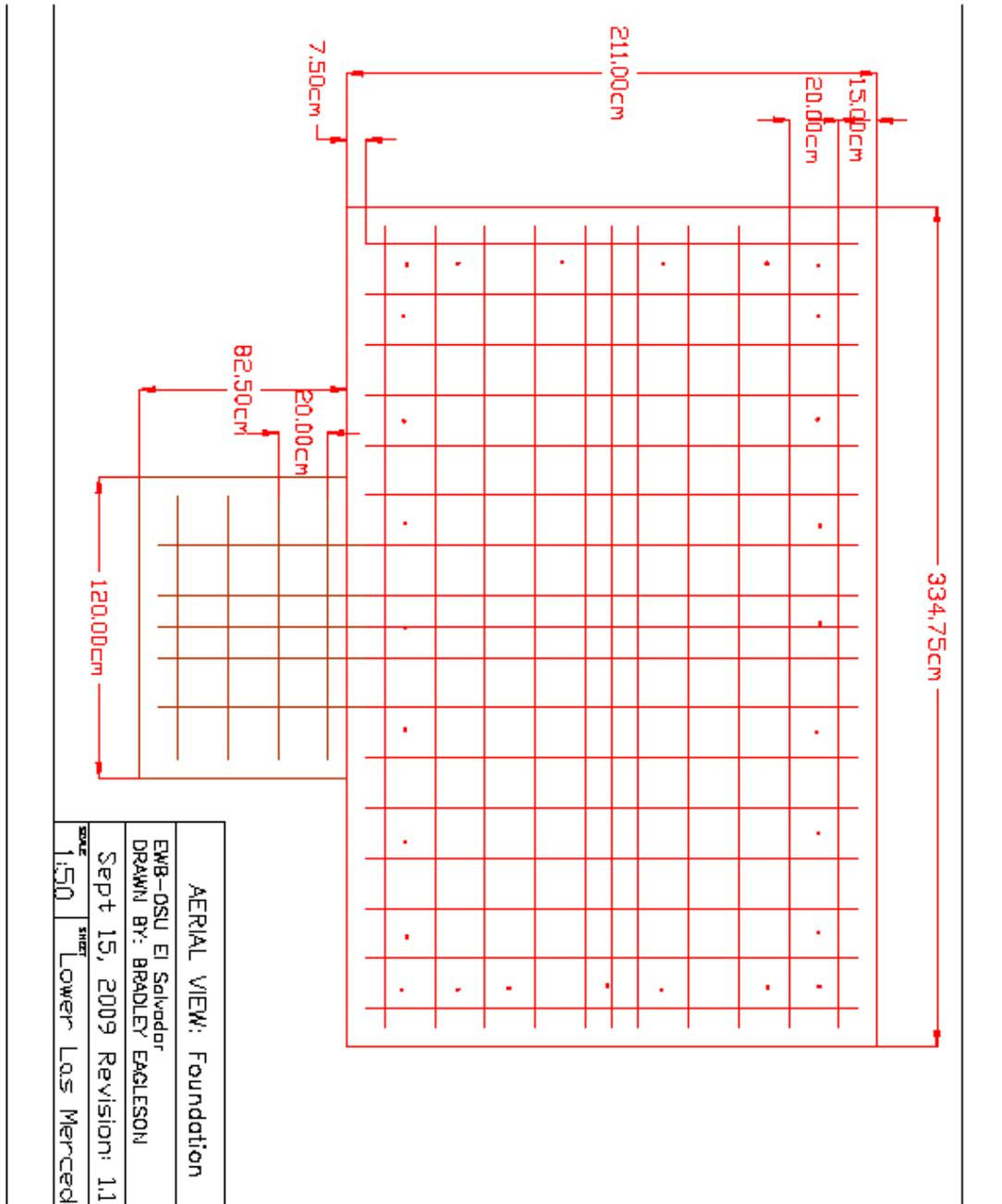
Figure 11: Foundation schematic drawn at 1:50 scale for the Lower Las Mercedes tank system. The small dots are locations of “L” hooks tied into the foundation.
