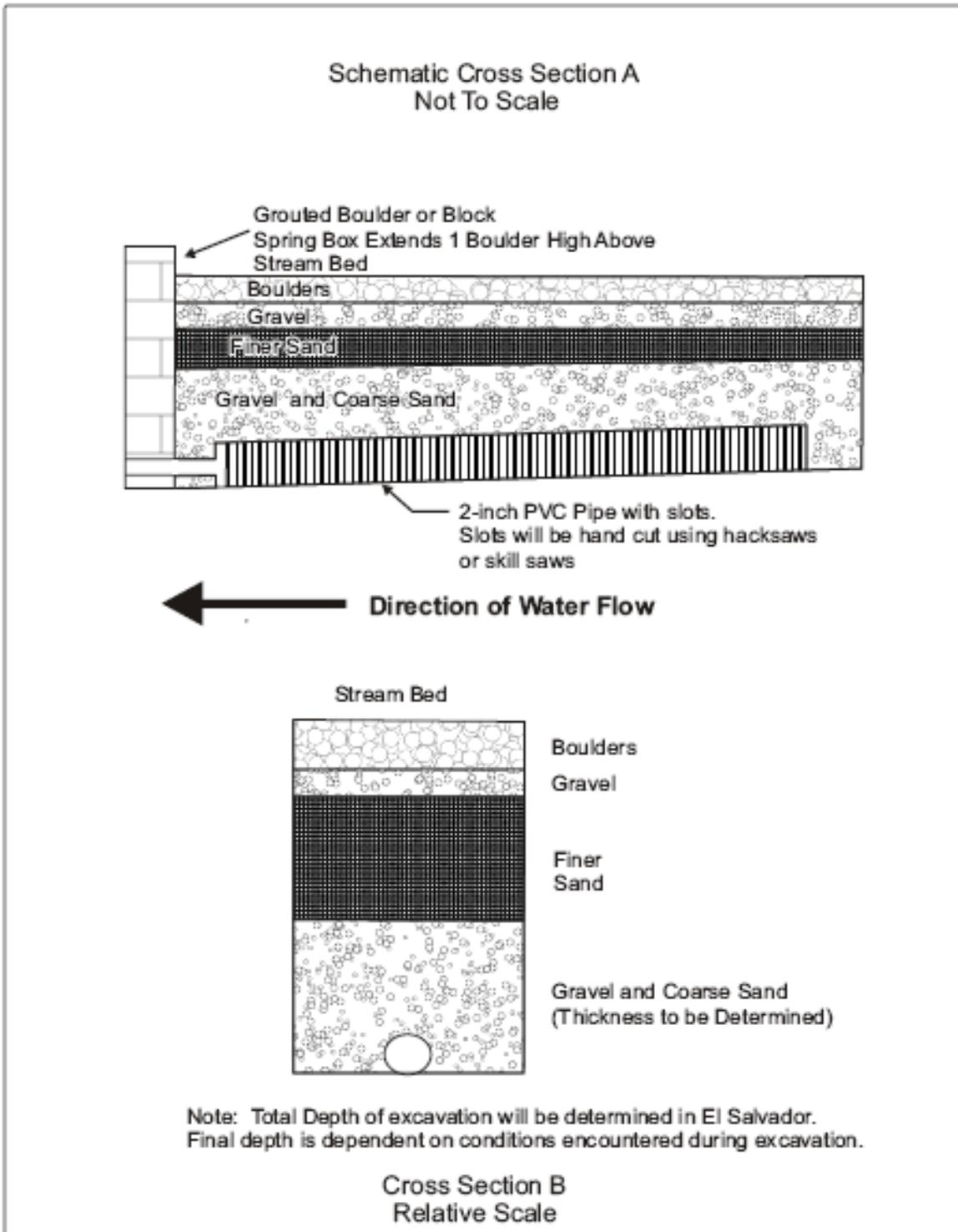
Fig. 10: Schematic drawing of the infiltration gallery. A nearly identical system was built in the community in June 2008.
