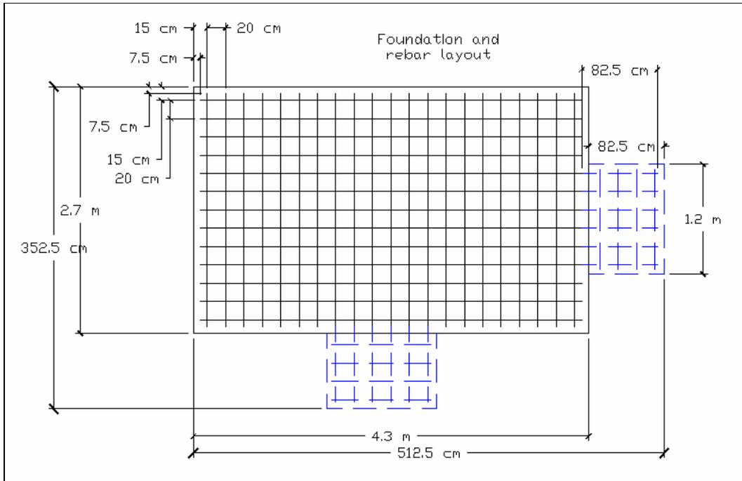
**Figure 8.B.1:** Tank foundation rebar layout- plan view
