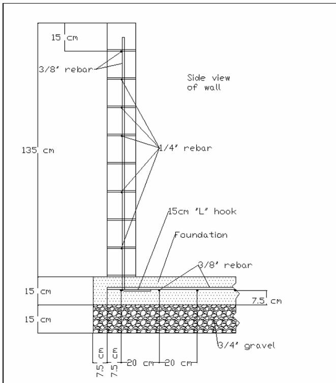
**Figure 8.B.2:** Tank foundation and side wall – profile view
