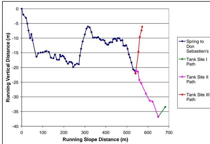
*Figure 5.2: Slope Distance vs. Elevation Change. Each potential tank location is shown. The large elevation increase at 300 m could be avoided by crossing through Don Eucelio Lopez's land.*
