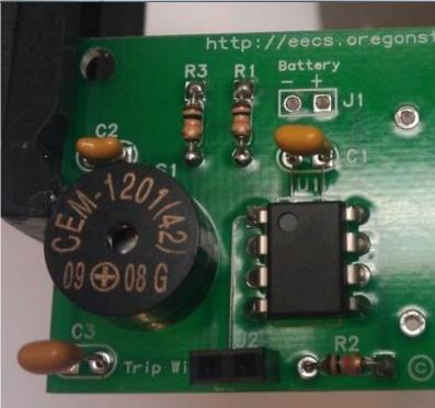
This step is just like the resistors. The capacitors are the same value. Put them in C1, C2, and C3. Bend the leads before flipping the PCB over. Solder and trim the leads.
