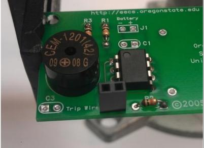
• Put the two pin female header in the spot marked J2. This is where the trip wire will be.
