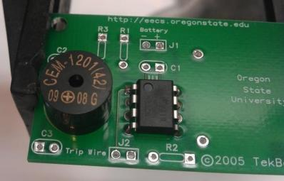
Place the Piezoelectric Buzzer as shown with the plus sign on the same side as the silk screening. The buzzer may need to be held when you flip the PCB over. Flip the board and solder.
