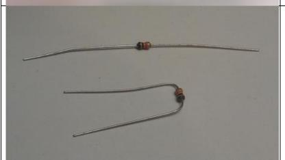
• Bend the resistor leads so they will fit into the holes.
