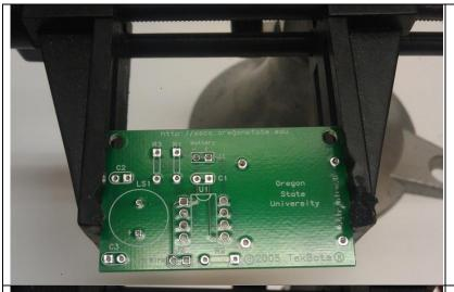
Place the PCB in the PCB vice with the top facing up. The top has the white silkscreened parts and words
