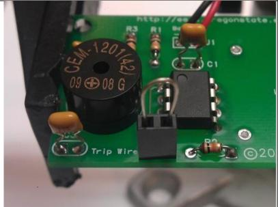
Take one of the cut leads and bend it so it fits into the female header. This will be pulled out by the trip wire and sound the alarm.
